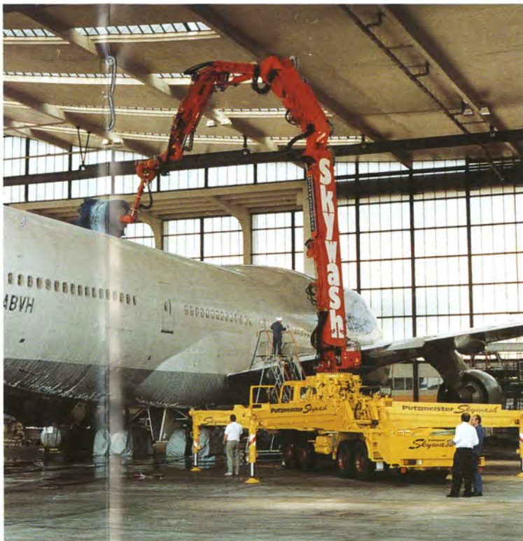
Washing the top of the fuselage, the multi-section boom keeps away from the ceiling of the hangar.
