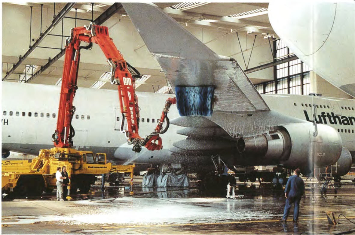
Skywash on Mercedes Benz truck with reduced emissions permits operation in closed hangars.
