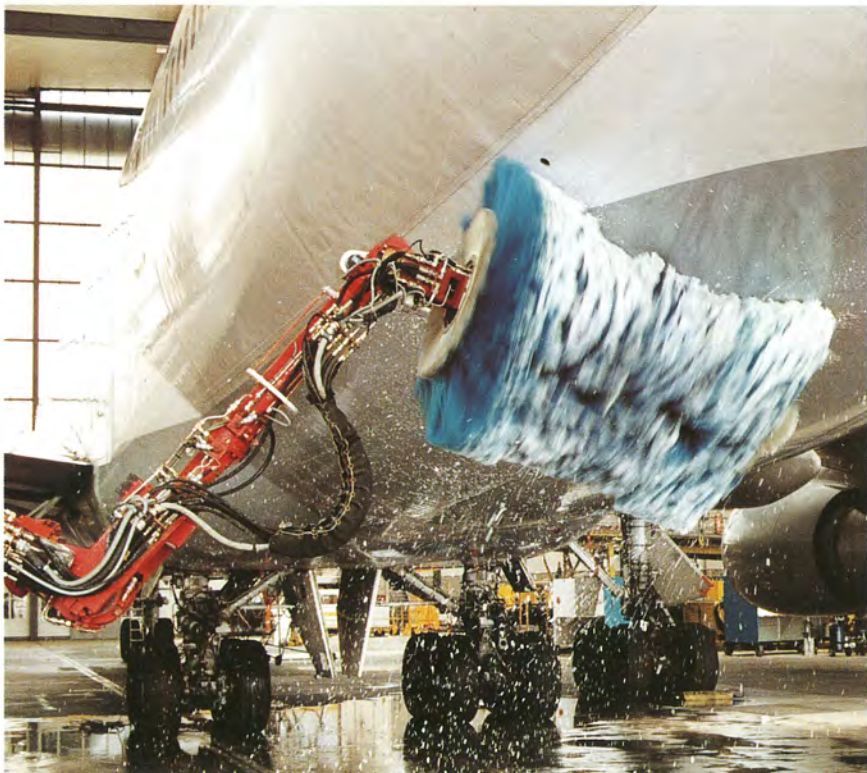
The sensor washing brush adapts to the rounded fuselage by defined centrifugal forces pressing the brush to the surface.
