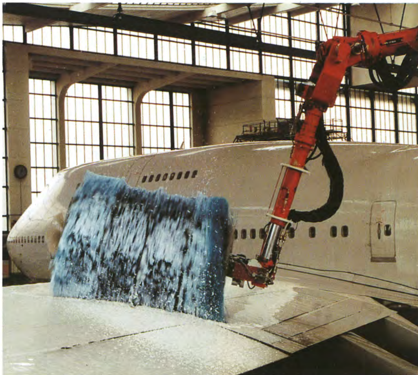
The washing brush compensates for geometric deviations of more than 1 metre.
